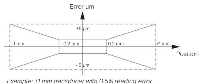
For standardised analogue transducers the error envelope is with respect to the nominal transducer sensitivity and therefore the total error includes both linearity and sensitivity errors. For non standardised transducers the error curve is with respect to the actual sensitivity and therefore any subsequent electronics will be required to adjust for the actual sensitivity of the transducer.
