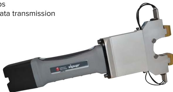
Multi Channel WiGauge™ used with narrow body probes to create a crank gauge
