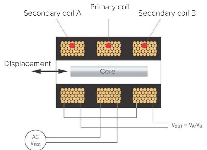
The output of an LVDT is a linear function of the displacement over its calibrated range. Beyond this range the output becomes increasingly non linear. Measurement range is defined as  $\pm$  distance from the transducer zero or null position.
