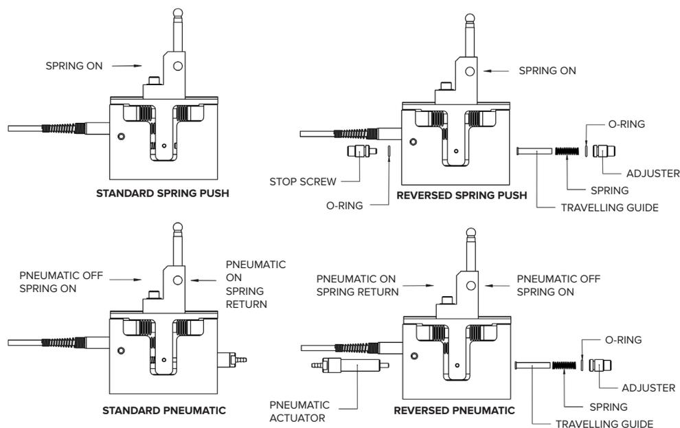
Spring and Pneumatic kits enable the automatic loading of components. Pneumatic actuation coupled with a spring controls the tip force for accurate measurements.
