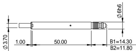
6 mm Diameter Body Gaiter Independent Pneumatic (A6J/P)
